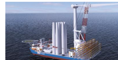
WTIV (Wind Turbine Installation Vessel)
